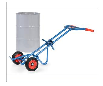
Welded tubular steel, powder-coated, RAL blue 5007, durable surface protection. Wheels with solid rubber tyres, hubs with roller bearings. Suitable for all rimmed 200 litre drums.
