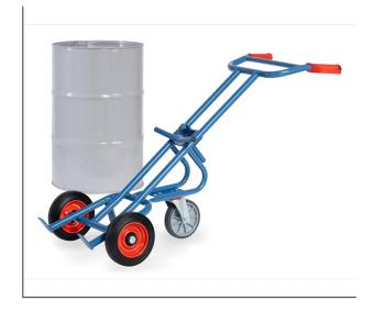
Welded tubular steel, powder-coated, RAL blue 5007, durable surface protection. Wheels with solid rubber tyres, hubs with roller bearings. Suitable for all rimmed 200 litre drums. Additional supporting castor wheel, TPE tyres 200 x 40 mm.
