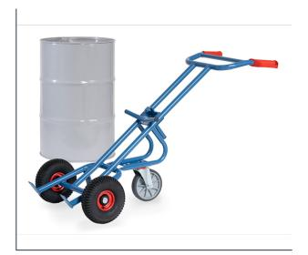
Welded tubular steel, powder-coated, RAL blue 5007, durable surface protection. Wheels with pneumatic tyres, hubs with roller bearings. Suitable for all rimmed 200 litre drums. Additional supporting castor wheel, TPE tyres 200 x 40 mm.
