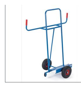
For longitudinal transport of bulky wooden boards and plastic sheets. Tubular steel construction with steel sheet blade, powder coated blue RAL 5007. Wheels with pneumatic tyres. Hubs with roller bearings. 2 support wheels 50 mm Ø. For the longitudinal transport of large-area wooden and plastic panels. Flat packed delivery.
