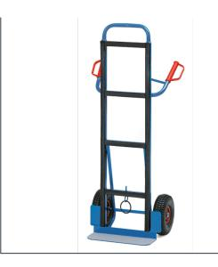
For transporting appliances, such as stoves, refrigerators, washing machines, etc. Welded tubular steel construction, powder coated in blue RAL 5007. Wide rubber pads and non-slip cover on the blades. Pneumatic tyres, wheel hubs with roller bearings.
