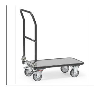
Tubular steel construction, powder coated anthracite grey, with platform made of derived timber material boards. Surface grey. Handlebar foldable onto platform. 2 swivel and 2 fixed-wheel castors, TPE tyres, hubs with groove ball bearing. Swivel castors with wheel locks, according to the European Standard EN 1757-3 (safety of platform trolleys).
