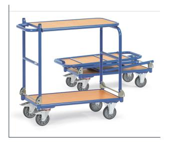
Tubular steel construction, powder coated, with platform made of derived timber material boards. Surface beech grain. 2 handlebars foldable onto platform. With additional foldable table platform. 2 swivel and 2 fixed-wheel castors, TPE tyres, hubs with groove ball bearing. Swivel castors with wheel locks, according to the European Standard EN 1757-3 (safety of platform trolleys).
