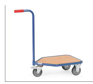
Made of tubular steel welded and powder coated, blue RAL 5007, with wooden platform, handles bolted on. 1 swivel castor and 2 fixed-wheel castors. Wheels with TPE tyres, hubs with precision deep grove ball bearing. Swivel castor with wheel locks, according to the European Standard EN 1757-3 (safety of platform trolleys).
