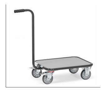
Made of tubular steel welded and powder coated, anthracite grey RAL 7016, with wooden platform, handles bolted on. 2 swivel castors and 2 fixed-wheel castors. Wheels with TPE tyres, hubs with precision deep grove ball bearing. Swivel castors with wheel locks, according to the European Standard EN 1757-3 (safety of platform trolleys).
