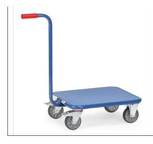
Made of tubular steel welded and powder coated, blue RAL 5007, with steel sheet platform, flush with frame, handles bolted on. 2 swivel castors and 2 fixed-wheel castors. Wheels with TPE tyres, hubs with precision deep grove ball bearing. Swivel castors with wheel locks, according to the European Standard EN 1757-3 (safety of platform trolleys).
