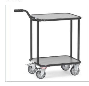
Made of tubular steel welded and powder coated, anthracite grey RAL 7016, with 2 wooden platforms, handles bolted on. 2 swivel castors and 2 fixed-wheel castors. Wheels with TPE tyres, hubs with precision deep grove ball bearing. Swivel castors with wheel locks, according to the European Standard EN 1757-3 (safety of platform trolleys). Capacity upper shelf 100 kg.
