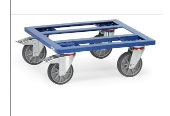
Frame made of angular steel, welded, powder coated, blue RAL 5007. With open frame. 4 swivel castors, wheels with TPE tyres, hubs with precision deep grove ball bearing. 2 swivel castors with wheel locks, according to the European Standard EN 1757-3 (safety of platform trolleys).
