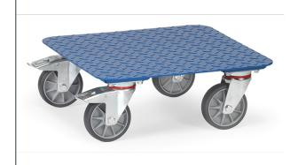
Welded construction with chequer plate platform, powder coated, blue RAL 5007. 4 swivel castors, wheels with TPE tyres, hubs with precision deep grove ball bearing. 2 swivel castors with wheel locks, according to the European Standard EN 1757-3 (safety of platform trolleys).
