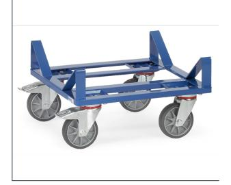
Frame made of angular steel, welded, powder coated, blue RAL 5007. With cradle for reels, bales etc. 4 swivel castors, wheels with TPE tyres, hubs with precision deep grove ball bearing. 2 swivel castors with wheel locks, according to the European Standard EN 1757-3 (safety of platform trolleys).
