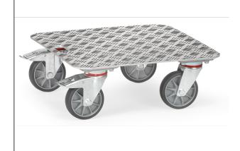
Welded construction with aluminium platform with ribbed structure. 4 swivel castors, wheels with TPE tyres, hubs with precision deep grove ball bearing. 2 swivel castors with wheel locks, according to the European Standard EN 1757-3 (safety of platform trolleys).
