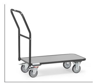
Tubular steel, welded construction, powder coated, anthracite grey RAL 7016. Platform made of derived timber material board, surface grey. 2 swivel and 2 fixed-wheel castors, TPE tyres, hubs with groove ball bearing. Swivel castors with wheel locks, according to the European Standard EN 1757-3 (safety of platform trolleys).
