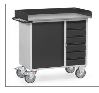
Made of steel sheets with 1 cupboard, 1 fixed and 2 adjustable shelves, and 6 drawers (H x W x D: 95 x 280 x 470 mm) with sliding guide. Centrally lockable by cylinder lock. Powder coated, carcass grey RAL 7035, front anthracite grey RAL 7016. Worktop composite panel grey 20 mm. 2 swivel and 2 fixed-wheel castors, TPE tyres, hubs with groove ball bearing. Swivel castors with wheel locks, according to the European Standard EN 1757-3 (safety of platform trolleys).
