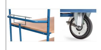
Compact and light wheel lock for all trolleys and carts with 2 swivel castors and standard TPE tyres up to 600 kg capacity. Actuation bar at push handle released: brake tightened, cart is safed against rolling away reliable. Actuation bar pushed: brake released, cart can be moved easily. Ergonomic and smooth operation. Safe braking effect due to formefitting disabling dovetailing. Not usable as driving brake. Surcharge per trolley. Can not be retrofitted.
