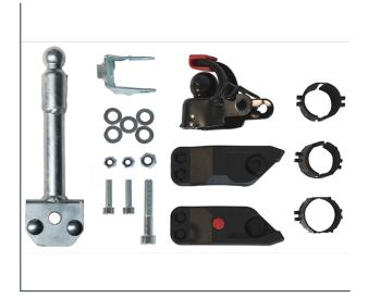
Mounting kit hot-dip galvanised consisting of ball coupling and adapter for seat posts with a diameter of 26 to 31 mm and bolt-on plates on standard drawbar. Load capacity max. 40 kg, fifth wheel load max. 4 kg. Can be retrofitted.
