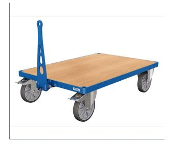
For transport with towing vehicles up to 6 km / h. Trains up to 5 cars possible. Maximum draw weight 2,000 kg. Tiller profiled from flat steel, automatically sets itself by means of gas springs in vertical rest position. There is a stable coupling pin on the castor side. Connection possible by foot control.
