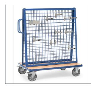
Sectional steel, with welded wire lattice 75 x 75 mm, powder coated, blue RAL 5007. Continuous platform of derived timber material board, surface beech grain. Wheels: 2 swivel and 2 fixed-wheel castors, TPE tyres, hubs with groove ball bearing. Swivel castors with wheel lock. Height of superstructure 1250 mm. Total height 1536 mm. Wire lattice frame inclined at 11%.
