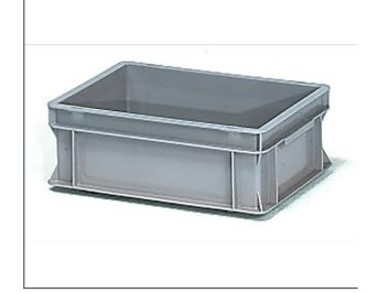
Made of high-quality, shock-resistant plastic, mainly Polyethylene (PE) and Polypropylene (PP). These materials are resistant to all common alkaline solutions and acids, neutral to smell and taste, physiologically recognized as safe and remain in the temperature range between - 40° and + 100° stable as far as dimensions and material is concerned. Colour grey, in standard Euro dimensions.
