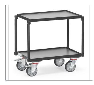
Compatible for Euro boxes 600 x 400 mm, powder coated anthracite grey RAL 7016. Roller with 2 platforms. Both platforms of derived timber material board middle grey housed in frames, rim 15 mm high. Clearance between platforms 390 mm, total height 630 mm. 4 swivel castors, TPE tyres, hubs with groove ball bearing. 2 swivel castors with wheel locks, according to European Standard EN 1757-3 (safety of platform trolleys). Flat packed delivery.
