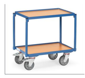
Compatible for Euro boxes 600 x 400 mm, powder coated blue RAL 5007. Roller with 2 platforms. Both platforms of derived timber material board housed in frames, rim 15 mm high. Clearance between platforms 390 mm, total height 630 mm. 4 swivel castors, TPE tyres, hubs with groove ball bearing. 2 swivel castors with wheel locks, according to European Standard EN 1757-3 (safety of platform trolleys). Flat packed delivery.
