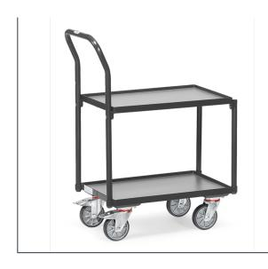
Compatible for Euro boxes 600 x 400 mm, powder-coated anthracite grey RAL 7016. Roller with 2 platforms. Both platforms of derived timber material board housed in frames, rim 15 mm high. Clearance between platforms 390 mm, total height 630 mm. 4 swivel castors, TPE tyres, hubs with groove ball bearing. 2 swivel castors with wheel locks, according to European Standard EN 1757-3 (safety of platform trolleys).
