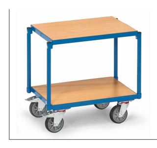
Compatible for Euro boxes 600 x 400 mm, powder-coated blue RAL 5007. Roller with 2 platforms. Both platforms of derived timber material board housed in frames, rim 10 mm high. Clearance between platforms 390 mm, total height 630 mm. Platforms flush with top edge of frame. 4 swivel castors, TPE tyres, hubs with groove ball bearing. 2 swivel castors with wheel locks, according to European Standard EN 1757-3 (safety of platform trolleys).
