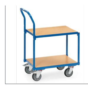
Compatible for Euro boxes 600 x 400 mm, powder-coated blue RAL 5007. Roller with 2 platforms. Both platforms of derived timber material board housed in frames, rim 10 mm high. Clearance between platforms 390 mm, total height 630 mm. 4 swivel castors, TPE tyres, hubs with groove ball bearing. 2 swivel castors with wheel locks, according to European Standard EN 1757-3 (safety of platform trolleys). Flat packed delivery.
