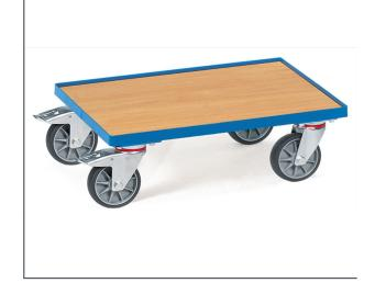
Suitable for Euro boxes, 600 x 400 mm, powder coated, blue RAL 5007. With platform made of derived timber boards, skirting 10 mm high. 4 swivel castors, TPE tyres. 2 swivel castors with wheel locks, according to the European Standard EN 1757-3 (safety of platform trolleys).
