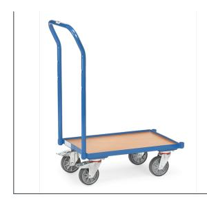
Suitable for Euro boxes,  $600 \times 400$  mm, powder coated, blue RAL 5007. With platform made of derived timber boards, skirting 10 mm high. 4 swivel castors, TPE tyres. 2 swivel castors with wheel locks, according to the European Standard EN 1757-3 (safety of platform trolleys).
