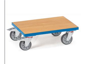
Suitable for Euro boxes, 600 x 400 mm, powder coated, blue RAL 5007. With platform made of derived timber boards, flush with frame. 4 swivel castors, TPE tyres. 2 swivel castors with wheel locks, according to the European Standard EN 1757-3 (safety of platform trolleys).
