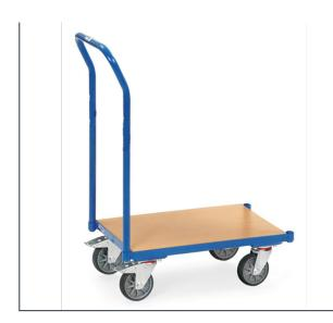
Suitable for Euro boxes, 600 x 400 mm, powder coated, blue RAL 5007. With platform made of derived timber boards, flush with frame. 4 swivel castors, TPE tyres. 2 swivel castors with wheel locks, according to the European Standard EN 1757-3 (safety of platform trolleys).
