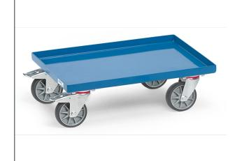
Suitable for Euro boxes, 600 x 400 mm, powder coated, blue RAL 5007. Steel plate tray leak-proof welded. Rim 22 mm high. Especially adapted for the transport of open-worked boxes with lubricated or wet parts. Nothing drips on the floor. 4 swivel castors, TPE tyres. 2 swivel castors with wheel locks, according to the European Standard EN 1757-3 (safety of platform trolleys).
