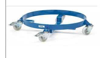
For upright transport of 60 litre or 200 litre steel drums. Welded steel construction, powder coated, blue RAL 5007. Interior-Ø 610 mm. 4 swivel castors, 2 with wheel lock. Wheels made of polyamide. Hubs with glide bearing.
