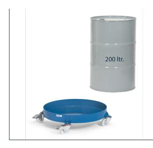
For upright transport of 200 litre steel drums. Welded steel construction, powder coated, blue RAL 5007. 4 swivel castors, 2 with wheel lock. Wheels made of polyamide. Hubs with glide bearing. With closed sheet steel save-pan, oil-proof welded. Interior-Ø 630 mm. Rim 80 mm high.
