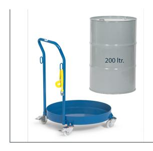
For upright transport of 200 litre steel drums. Welded steel construction, powder coated, blue RAL 5007. 4 swivel castors, 2 with wheel lock. Wheels made of polyamide. Hubs with glide bearing. With closed sheet steel save-pan, oil-proof welded. Interior-Ø 630 mm. Rim 80 mm high. Handle screw-on type, with 2 eyelets and 1 clamping band.
