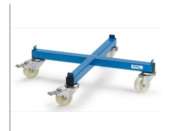
For upright transport or storage of 200 litre steel drums. Welded cross made of square pipe, with anti-slip corners, powder coated blue RAL 5007. 4 swivel castors, 2 with wheel lock, polyamide wheels, hubs with glide bearing.
