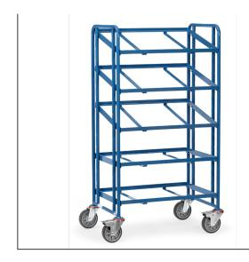
Modular system: Tubular and sectional steel construction, bolted, powder coated blue RAL 5007. Variable use of shelf frames, distance 150 mm, angle when inclined 15° and 30°. 5 shelf-frames for 3 Euro boxes each 600 x 400 mm. Delivery without boxes. 4 swivel castors with TPE tyres, hubs with groove ball bearing. 2 Swivel castors with wheel locks, according to European Standard EN1757-3 (safety of platform trolleys). Capacity upper and middle shelves 80 kg.
