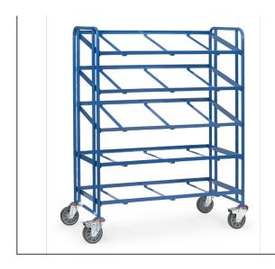
Modular system: Tubular and sectional steel construction, bolted, powder coated blue RAL 5007. Variable use of shelf frames, distance 150 mm, angle when inclined 15° and 30°. 5 shelf-frames for 3 Euro boxes each 600 x 400 mm. Delivery without boxes. 4 swivel castors with TPE tyres, hubs with groove ball bearing. 2 Swivel castors with wheel locks, according to European Standard EN1757-3 (safety of platform trolleys). Capacity upper and middle shelves 80 kg.
