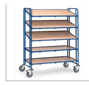
Modular system: Tubular and sectional steel construction, bolted, powder coated blue RAL 5007. Variable use of shelf frames, distance 150 mm, angle when inclined 15° and 30°. With 5 platforms made of derived timber material boards, rim 10 mm high. 4 swivel castors with TPE tyres, hubs with groove ball bearing. 2 Swivel castors with wheel locks, according to European Standard EN1757-3 (safety of platform trolleys). Capacity upper and middle shelves 80 kg.
