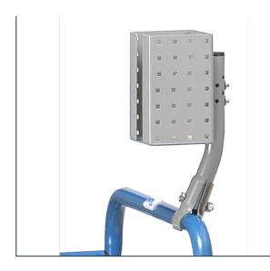
Steel sheet, powder coated in RAL 7035, with adjustable bolt-on points at the back and sides. Tubular strut with multiple holes, with clamping bracket for attaching the scanner bag onto almost all of our products in virtually any position. Scanner intake W x D x H:  $120 \times 87 \times 150$  mm Front opening: 40 mm wide.
