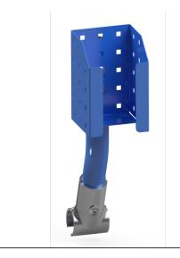
Sheet steel holder for disinfectant bottles, supplied as a building kit. Powder-coated blue RAL 5007. With variable screw-on points on the back and sides. Tube strut perforated many times, can be positioned as required with a clamp for fastening the holder. For standard Bode bottles with 500 ml content. Bottles not included in the delivery.
