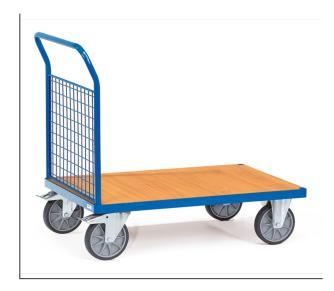
Tubular steel and profile steel welded, powder coated, surface durably protected, resistant to impact and scratches. Platform made of derived timber material boards, surface beech grain. Ends made of wire lattice 50 x 50 x 4 mm. Height of end panel 500 mm. 2 swivel and 2 fixed-wheel castors, TPE tyres, hubs with groove ball bearing. Swivel castors with wheel locks, according to the European Standard EN 1757-3 (safety of platform trolleys).
