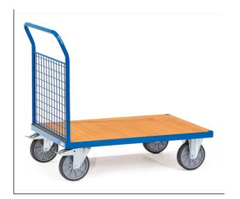
Tubular steel and profile steel welded, powder coated, surface durably protected, resistant to impact and scratches. Platform made of derived timber material boards, surface beech grain. Ends made of wire lattice 50 x 50 x 4 mm. Height of end panel 500 mm. 2 swivel and 2 fixed-wheel castors, TPE tyres, hubs with groove ball bearing. Swivel castors with wheel locks, according to the European Standard EN 1757-3 (safety of platform trolleys).
