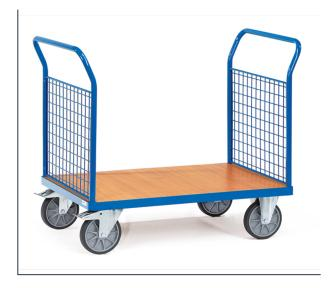
Tubular steel and profile steel welded, powder coated, surface durably protected, resistant to impact and scratches. Platform made of derived timber material boards, surface beech grain. Ends and made of wire lattice 50 x 50 x 4 mm. Height of end panel 500 mm. 2 swivel and 2 fixed-wheel castors, TPE tyres, hubs with groove ball bearing. Swivel castors with wheel locks, according to the European Standard EN 1757-3 (safety of platform trolleys).
