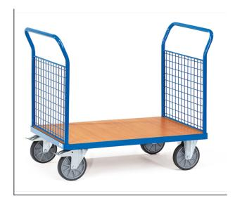
Tubular steel and profile steel welded, powder coated, surface durably protected, resistant to impact and scratches. Platform made of derived timber material boards, surface beech grain. Ends and made of wire lattice  $50 \times 50 \times 4$  mm. Height of end panel 500 mm. 2 swivel and 2 fixed-wheel castors, TPE tyres, hubs with groove ball bearing. Swivel castors with wheel locks, according to the European Standard EN 1757-3 (safety of platform trolleys).
