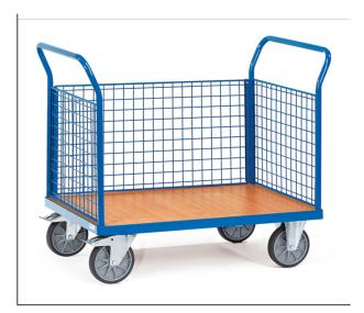
Tubular steel and profile steel welded, powder coated, surface durably protected, resistant to impact and scratches. Platform made of derived timber material boards, surface beech grain. Ends and 1 side made of wire lattice 50 x 50 x 4 mm. Height of end and side panel 500 mm. 2 swivel and 2 fixed-wheel castors, TPE tyres, hubs with groove ball bearing. Swivel castors with wheel locks, according to the European Standard EN 1757-3 (safety of platform trolleys).
