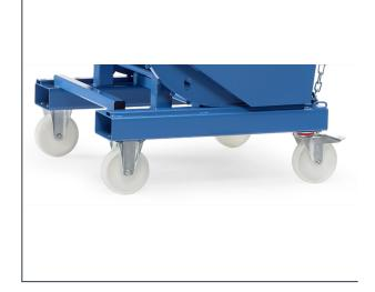
2 swivel and 2 fixed-wheel castors made of polyamide, size 200 x 50 mm, fitted underneath the fork-lift sleeves. Swivel castors with wheel locks, according to the European Standard EN 1757-3 (safety of platform trolleys).
