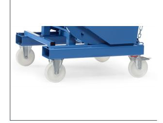
2 swivel and 2 fixed-wheel castors made of polyamide, size 200 x 50 mm, fitted underneath the fork-lift sleeves. Swivel castors with wheel locks, according to the European Standard EN 1757-3 (safety of platform trolleys).
