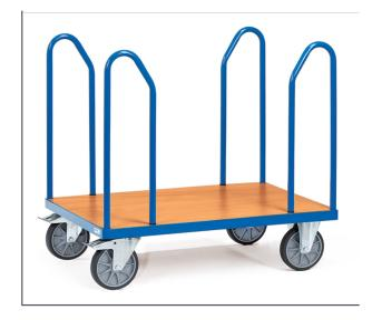
Tubular steel and profile steel welded, powder coated, surface durably protected, resistant to impact and scratches. Platform made of derived timber material boards, surface beech grain. With 4 high side frames. Height of side frames 750 mm. 2 swivel and 2 fixed-wheel castors, TPE tyres, hubs with groove ball bearing. Swivel castors with wheel locks, according to the European Standard EN 1757-3 (safety of platform trolleys).
