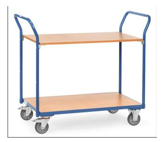
Modular system, platform and pushbar with screw connection, upper shelves can be inserted. Capacity upper shelf 80 kg. Disassembled on delivery. Welded tubular or sectional steel construction, powder coated, blue RAL 5007. Shelves made of derived timber material board, beech decor surface. 2 swivel and 2 fixed-wheel castors, TPE tyres, hubs with groove ball bearing. Swivel castors with wheel locks, according to the European Standard EN 1757-3 (safety of platform trolleys).
